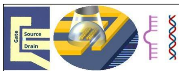
Figure 1: Merging of the plasmonic nanoparticles with the FET biosensor for the amplified response.
