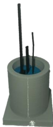
Figure 1: Electrochemical cell with incorporated electrodes, fabricated using FDM.
